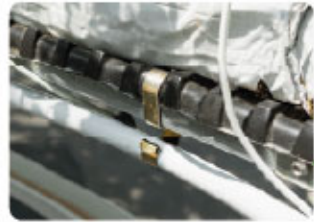
Hose clips specially designed for lateral irrigation
