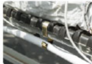
Hose clips specially designed for lateral irrigation
