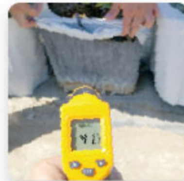
Pot temperature with cooling skirt raised.
