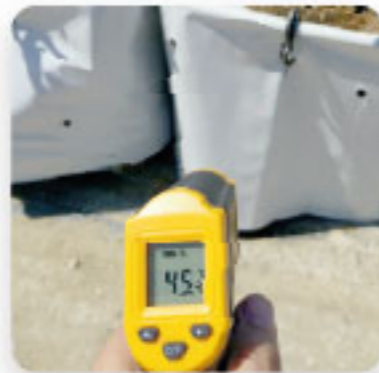
Pot temperature with cooling skirt.
